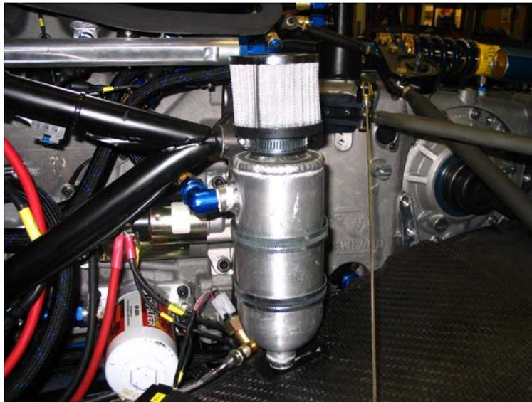
9. Install the exhaust assembly. Use the threaded rod and folded tag included in the kit to support the exhaust collector via the floor stay bracket on the LHS rear face of the tub. Remove the O<sup>2</sup> sensor from the rear-exit exhaust assembly and install in the side-exit exhaust assembly. Plug the O<sup>2</sup> sensor into the re-located wiring harness. Slide the inner half of the exhaust exit panel over the tail pipe with the return facing inboard (picture shown on step 17).
