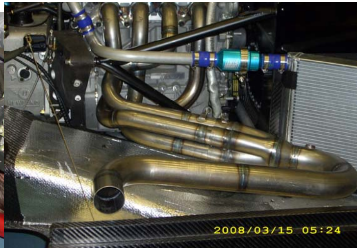
Engine Compartment & Rear Floor Stay RHS; Forward / Rear Primary DP02-60-079/080; Tail Pipe DP02-60-075
