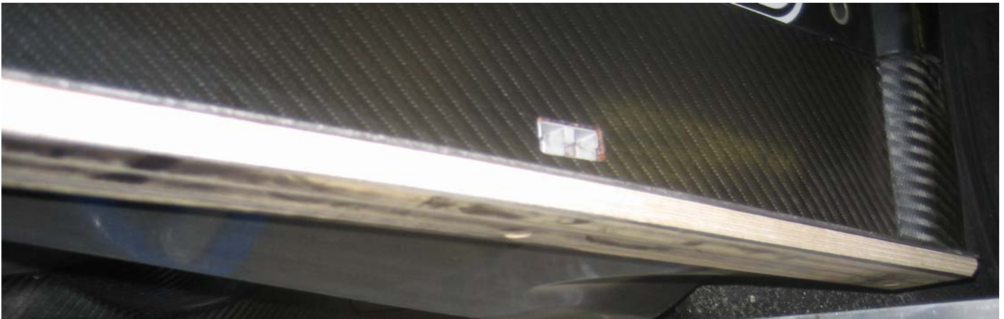
Tunnel Floor Outboard Rub Strip
