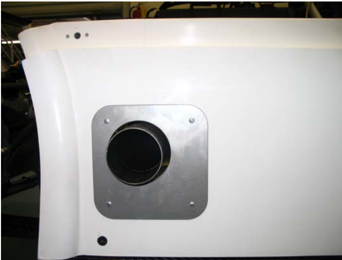
Exhaust Exit Location
