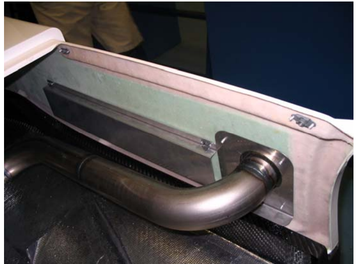
Exhaust Heat Shield & Exit Location
